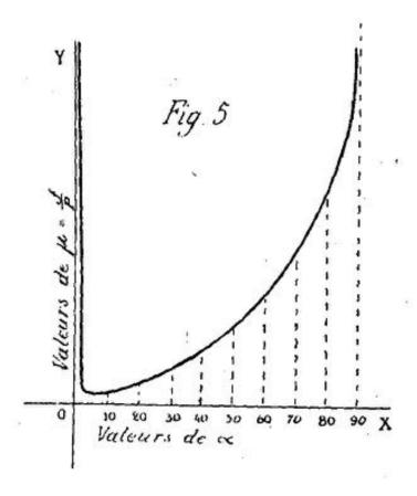
This minimum value for  $\alpha$ , neighboring 2 ° was determined by us in an earlier study from 1887, Therefore, based on the formulas of Duchemin, we calculate the different impacts under which a square meter of the load-bearing surface could hold a given weight in the air, advancing horizontally with a determined speed; then we drew up a table, of eight columns, in which each column corresponded to a bearing weight of 1,2,3 .... 8 kil. The horizontal
