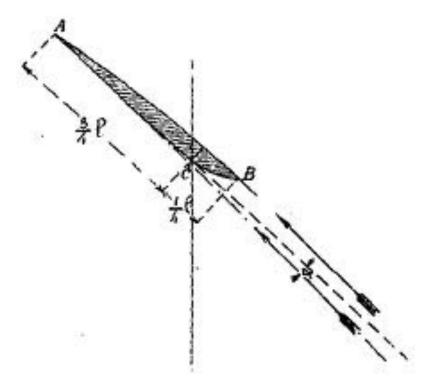
We can also adopt this same wing section, when the wing is not made of solid wood. It is possible to fix on the main beam, whether of wood or metal tube, transverse chords having the same section as that shown in figure 11, and spaced at a distance from each other along the radius, so as to form the helical surface of the wing. On these chords one would tend, on both sides of the wing, either a
