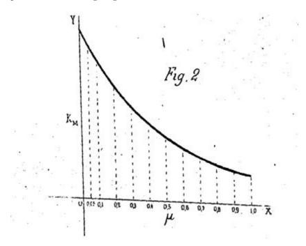
Let us draw the curve of the values of  $K_M$ , by varying  $\mu$  from 0 to 1, by increases of 0.1 (fig. 2). The ordinates of this curve are entered in the table below (Table A) below the corresponding values of  $\mu$  and the corresponding values  $\alpha$ . We see that  $K_M$  decreases very rapidly with the increase of  $\mu$  and that it is, there-fore, extremely important for the thrusters, as  $\mu$ , and hence also  $\alpha$ , are as small as possible.
