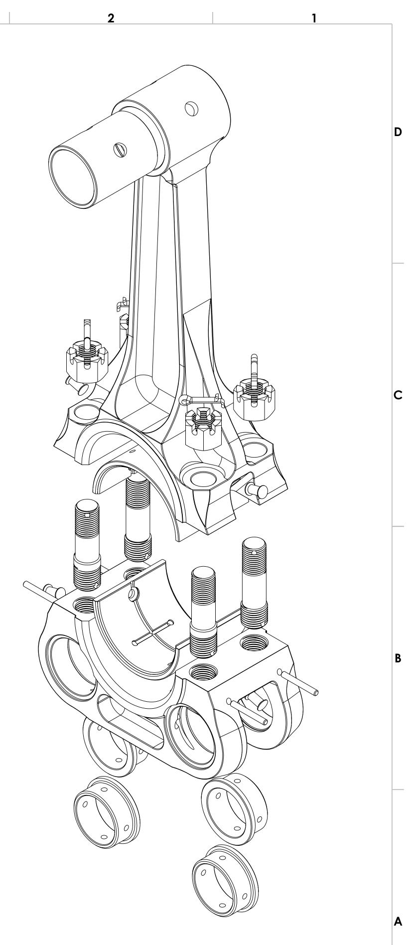
C-10039 Master Conn Rod Assy C-10016 Articulated Conn Rod Assy Master Rod assy use in production R-600 engines J Riend 31oct22
