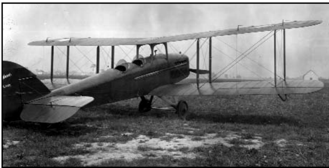
Packard's de Havilland DH-4C. Note the characteristic "Packard" upper wing-to-fuselage struts. The plane had a 1A-1237 engine installed and the tail marked "Packard Airplane" in the same manner as they marked their 1919 airplane. Courtesy NAHC collection.
