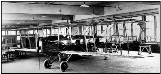
Packard airplane pictured in February of 1919 still on the factory floor. Note the shape of the upper wing to fuselage struts. This shape has only been noted on Packard-built or rebuilt airplanes. Courtesy Peter Bowers.
