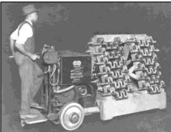
A smartly dressed Duesenberg worker transporting 24 King-Bugatti crankshaft halves, enough for six engines.
