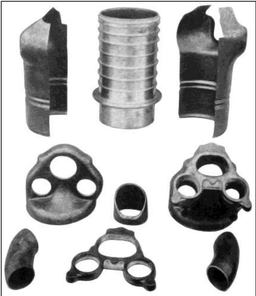
The steel stampings of the water jacket with the finished cylinder barrel in between, and the steel stampings that made up the cylinder head.
