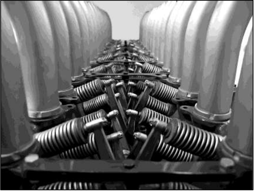
Another look at the 48 rocker arms exuding a level of elegance, sophistication, and complication that is not seen in modern engines (Martt Clupper photo via AirPigz, www.airpigz.com ).
