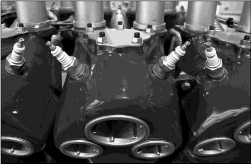
Close up view of the cylinder top. Note the water jacket welds and the overlapping lugs that tie the adjacent cylinders together on the right. The plate on the top of each cylinder is where the intake manifold would attach (Martt Clupper photo via AirPigz, www.airpigz.com ).
