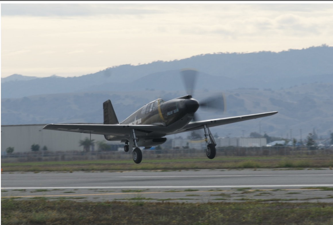
Pilot Dave Morss makes the first takeoff with Polar Bear fitted with the new 4-blade MT Propeller.
