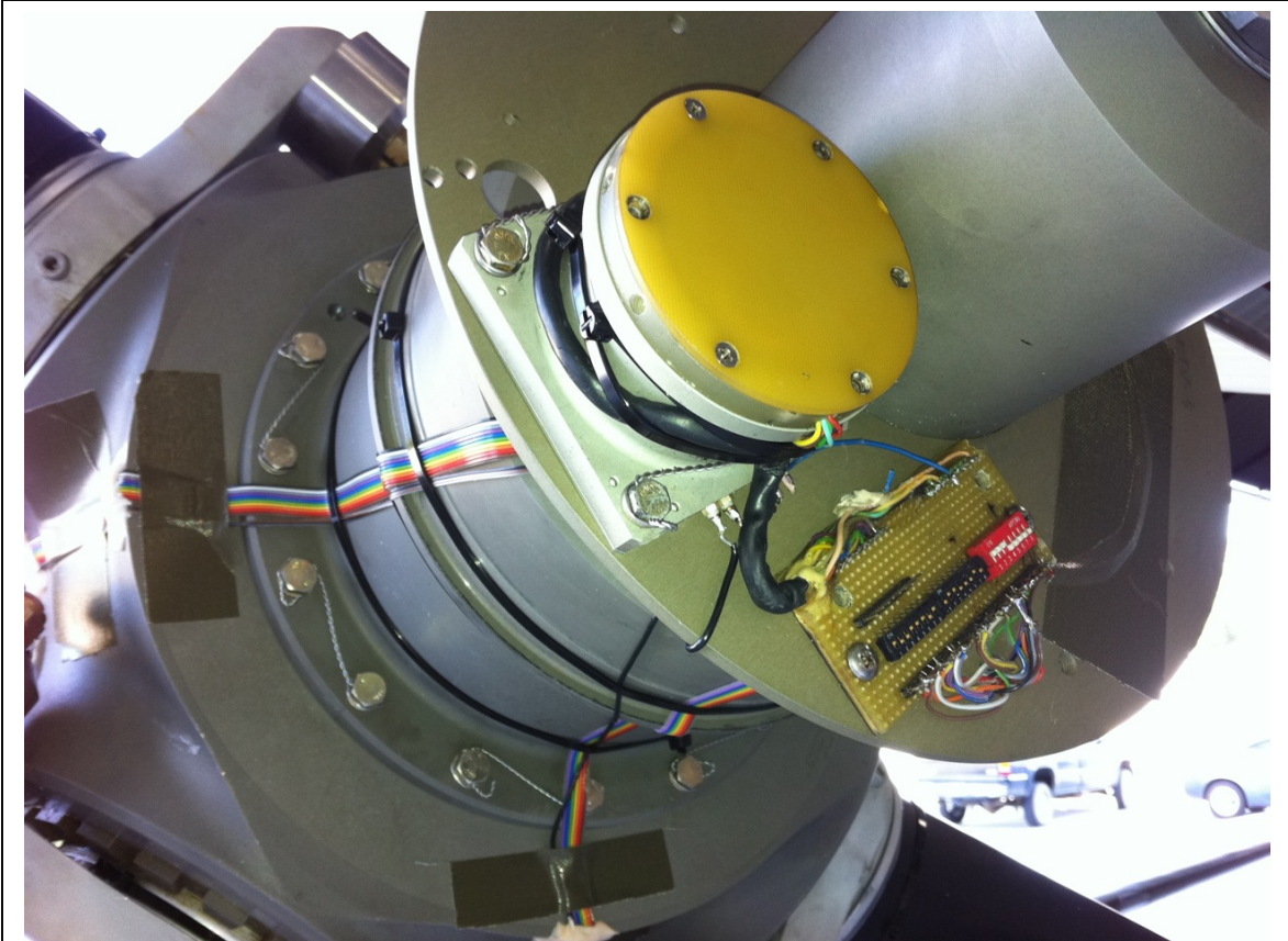
Here the wireless transmitter and stress measuring instruments are shown mounted on the hub before the spinner is installed.
