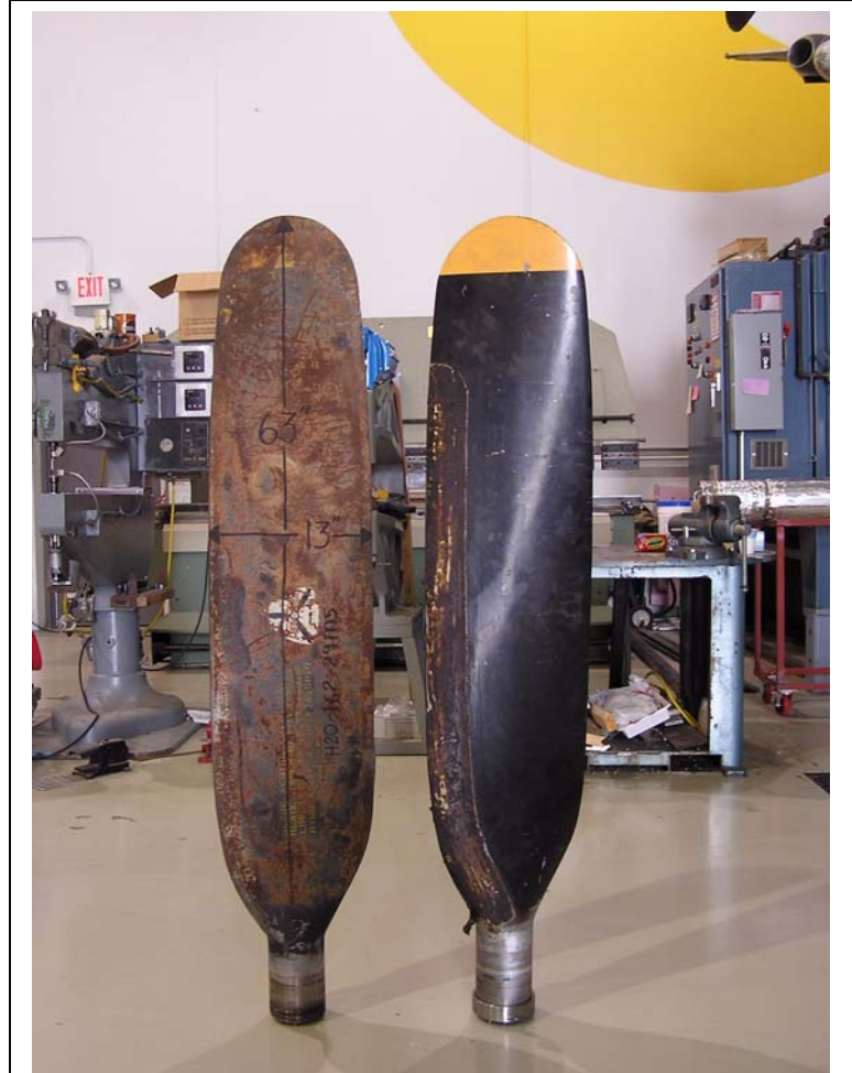
These original Aeroproducts blades are what the C & P Aviation team had to start with for propellers. The idea of finding serviceable propellers was attractive, and nearly became a showstopper for the restoration.
