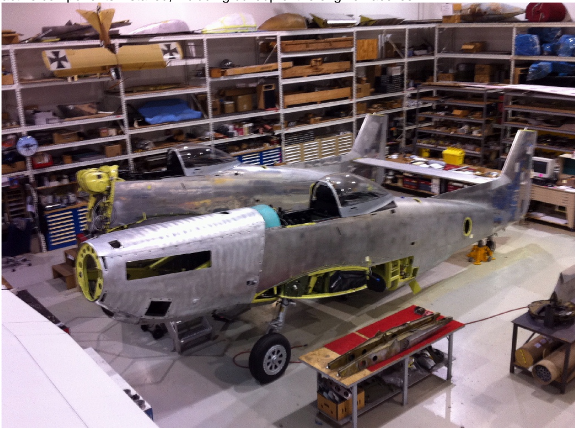
Current Status of P-82E #46-256. It's up on its wheels, wired and plumbed, and having system active components installed, including buildup of the engine nacelles.
