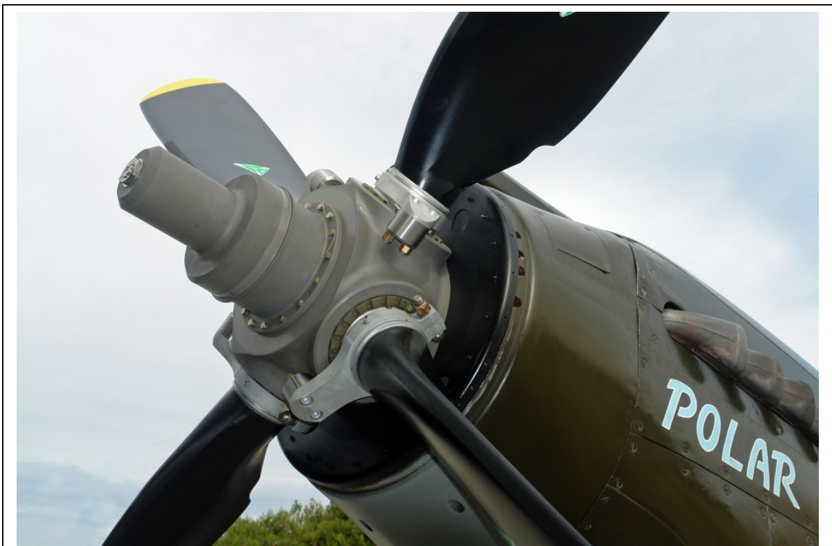
Another view of the propeller detailing the hub, blade attachment, counterweights and backing plate for the spinner. The profile of the trailing edge cutouts is clear as well.
