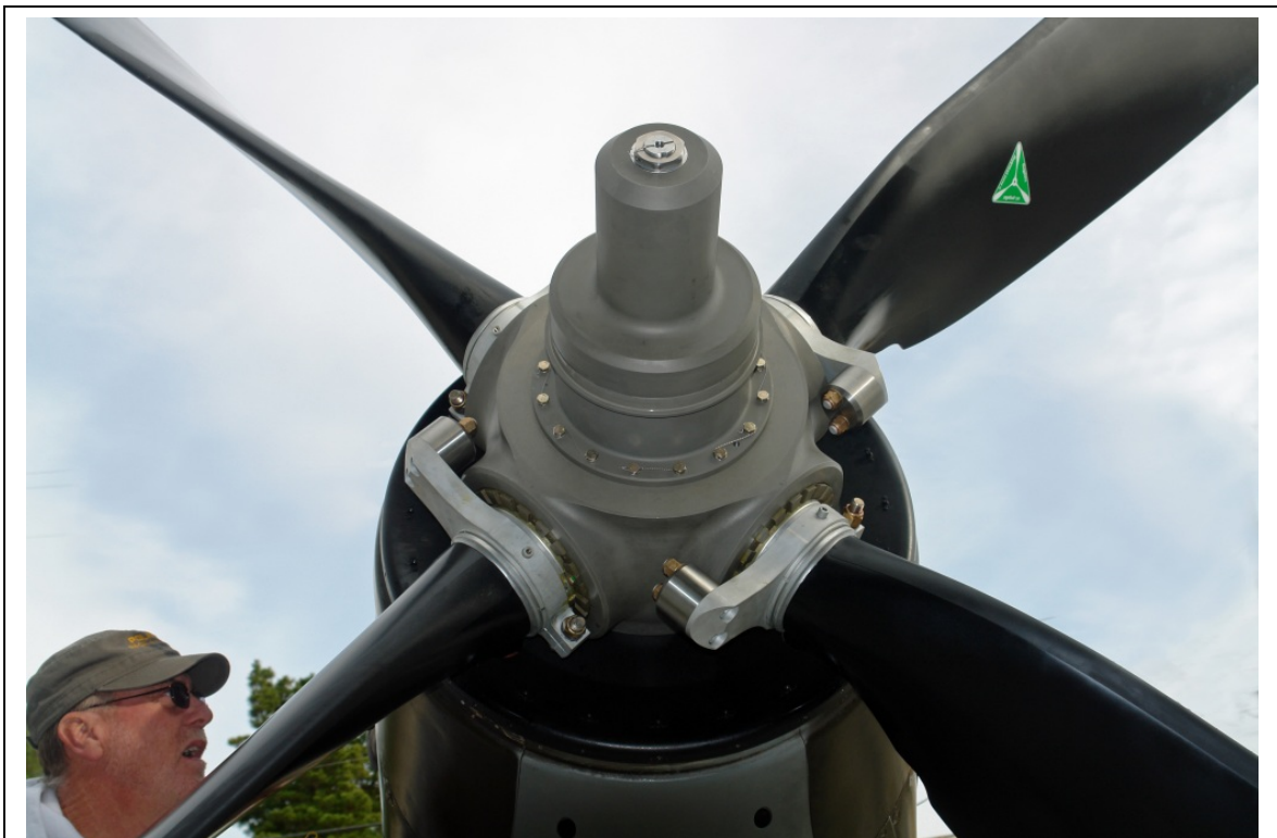
Dave Morss inspecting the propeller installation prior to first flight. Here the billet aluminum hub is very easy to see, as are the counterweights that assist in positioning the blades.
