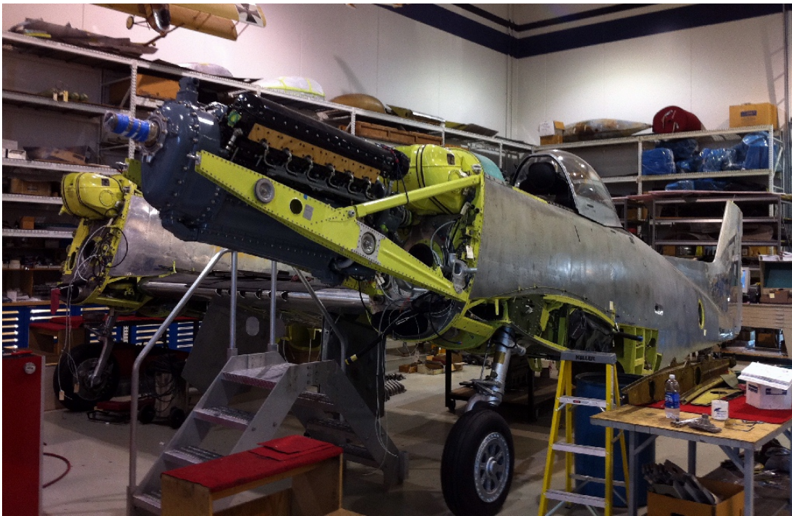
Current Status of P-82E #46-256. It's up on its wheels, wired and plumbed, and having system active components installed, including buildup of the engine nacelles.
