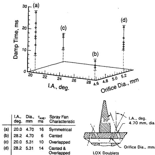
Fig. 13 Effect of near-wall modifications on stability characteristics of PFRT unit F1002.
