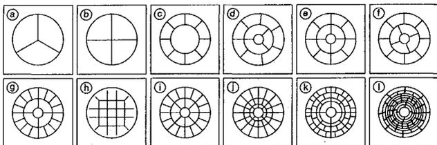
Fig. 3 Baffle patterns investigated during the F-1 Project First program.
