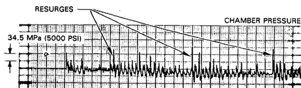
Fig. 7 Pressure trace exhibiting the resurge phenomena observed during bomb-induced perturbations of injector unit 076 with enlarged fuel orifices.
