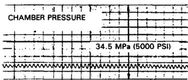
Fig. 12 Pressure trace exhibiting typical buzzing observed during the FRT and flight qualification development periods.
