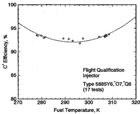
Fig. 19 Effect of fuel temperature on the flight qualification injector (type 5885).
