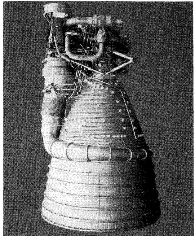
**Fig. 1 Key external features of the F-1 engine.**
