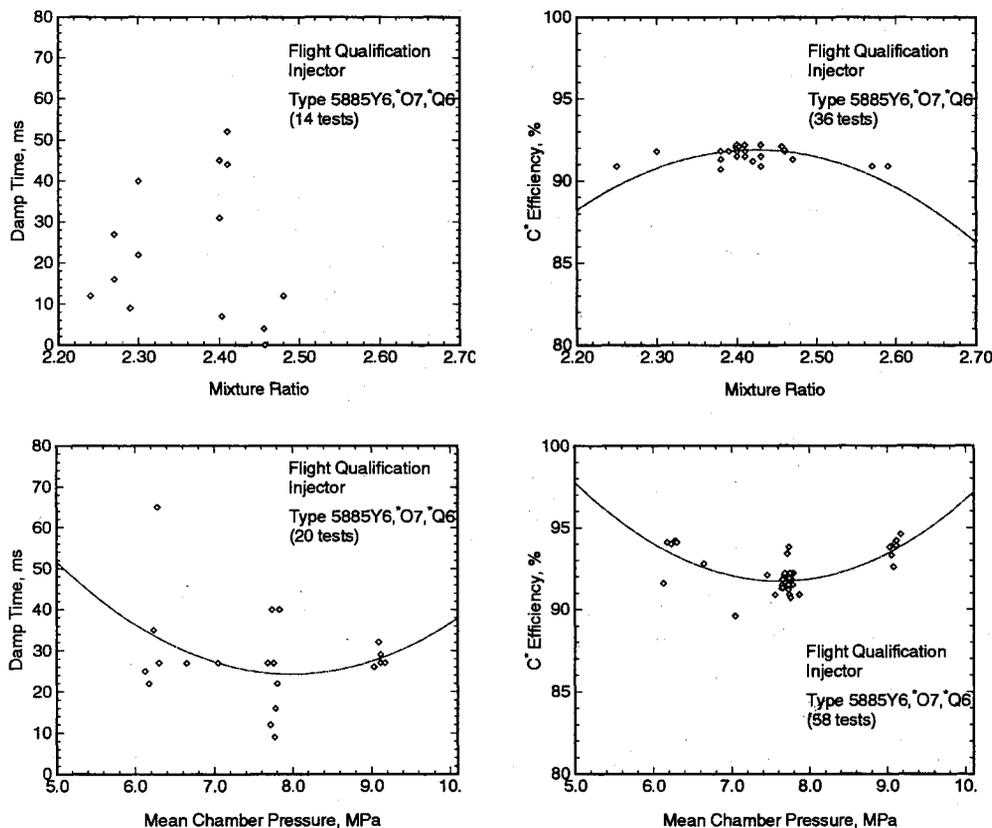
Fig. 18 Results of limits study conducted on the flight qualification injector (type 5885).
