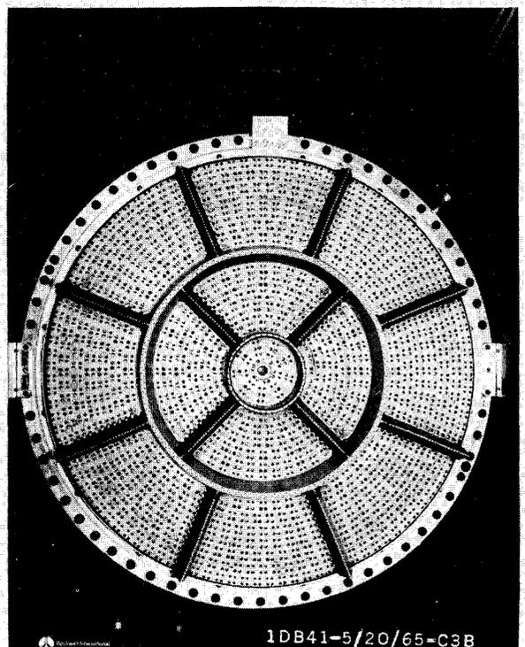
**Fig. 14 FRT injector configuration.**
