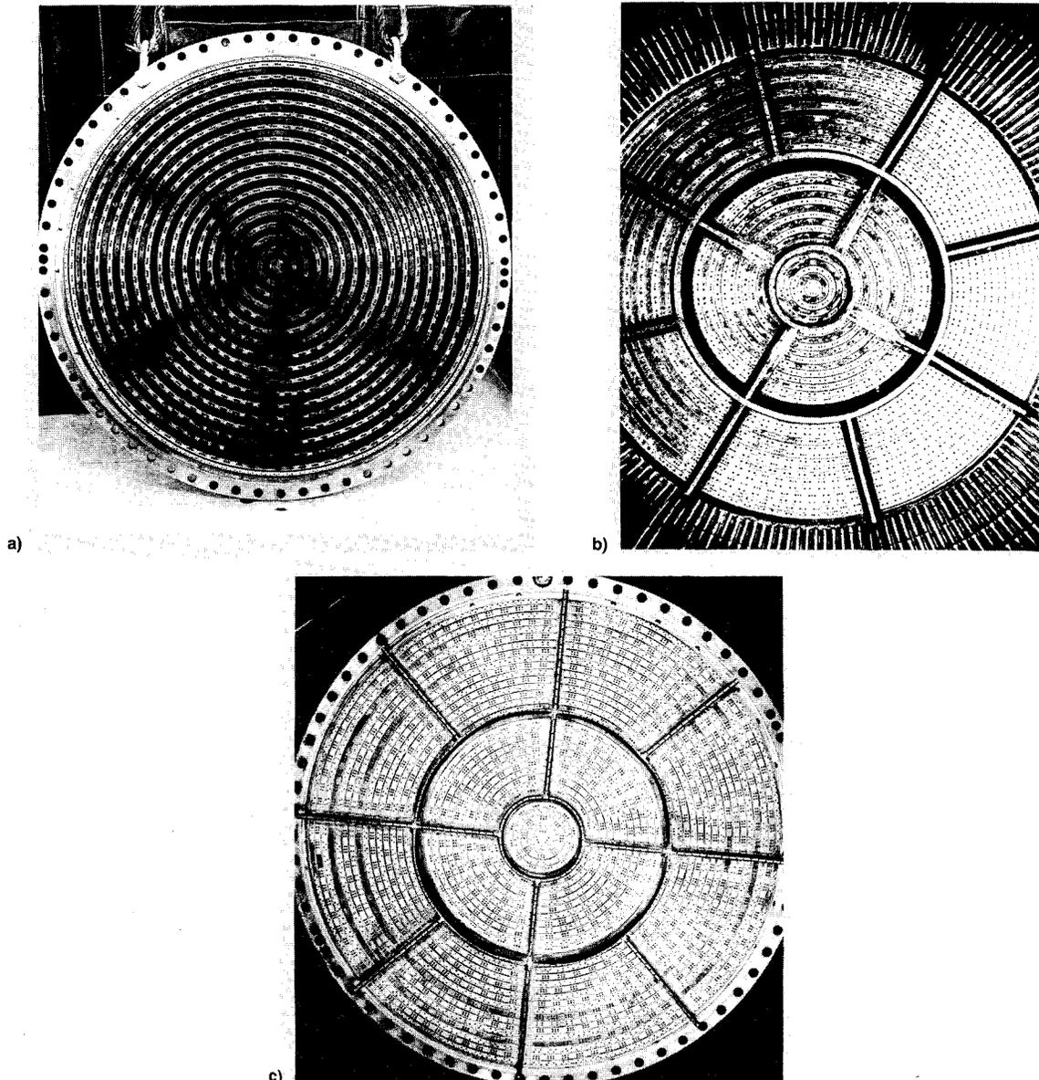
Fig. 4 Baseline injectors: a) 5U-flatface (unit 005, type 4852); b) 5U-baffled (unit 076, type 4866); and c) double-row cluster (unit 067, type 4838).
