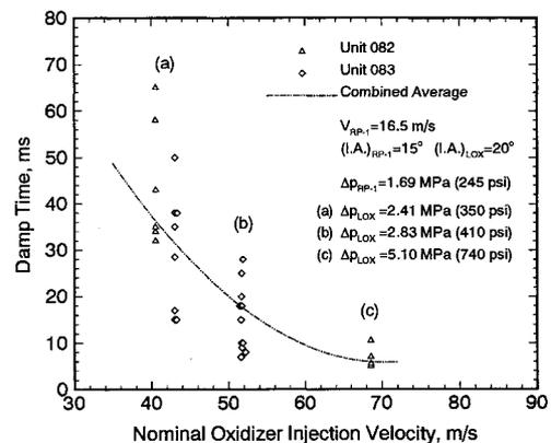
**Fig. 10 Damp time vs oxidizer injection velocity for tests conducted with injector units 082 and 083.**
