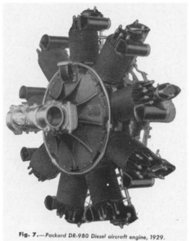
Fig. 7.—Packard DR-980 Diesel aircraft engine, 1929.
