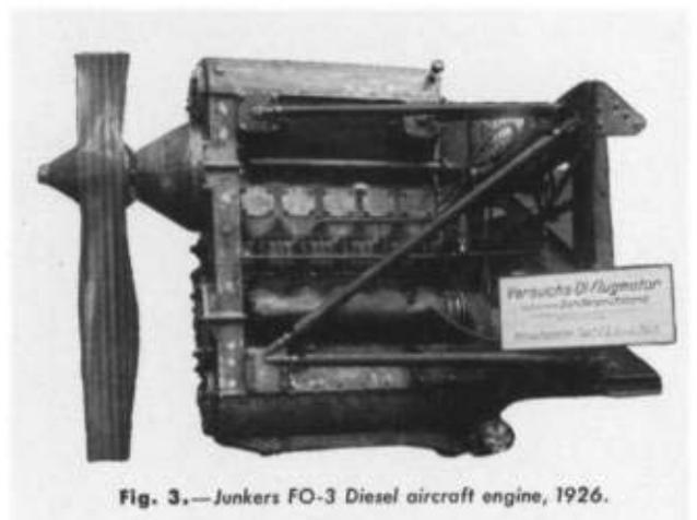
Fig. 3.—Junkers FO-3 Diesel aircraft engine, 1926.
