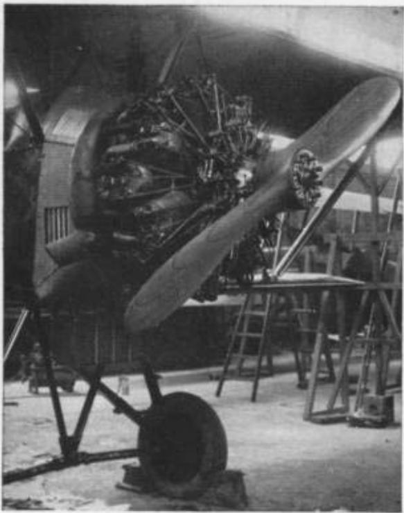
Fig. 14.—Clerget 14 F-01 Diesel aircraft engine, 1937.
