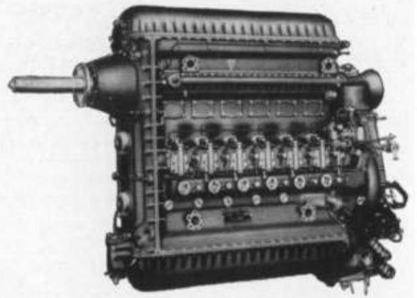
Fig. 4.—Junkers Jumo 205 Diesel aircraft engine, 1935-1939.
