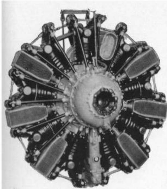
Fig. 5.—B.M.W.-Lanova 114 V-4 Diesel aircraft engine, 1938.
