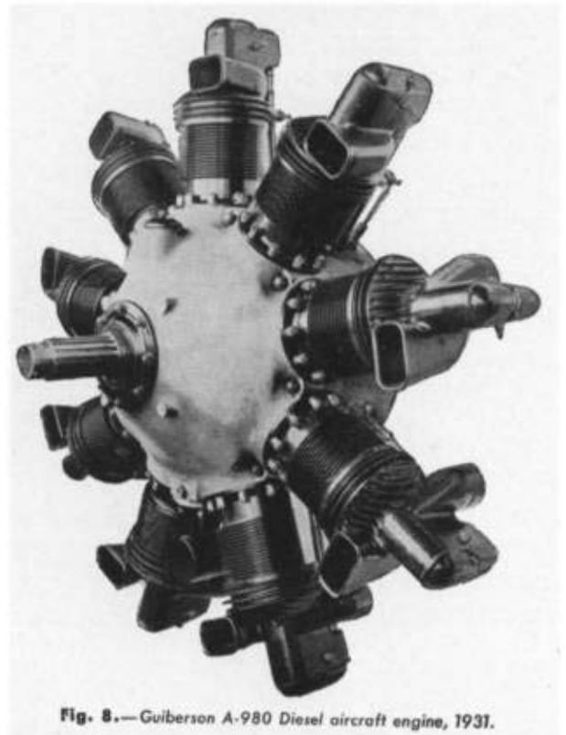
Fig. 8.—Guiberson A-980 Diesel aircraft engine, 1931.
