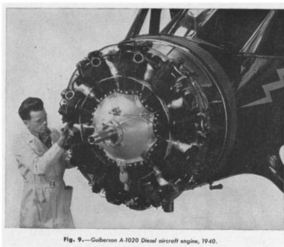
Fig. 9.—Guiberson A-1020 Diesel aircraft engine, 1940.
