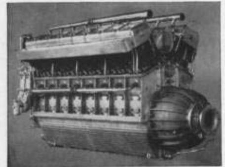
Fig. 6.—Mercedes-Benz DB 602 Diesel airship engine, 1936.
