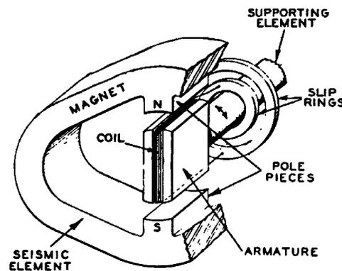
Figure 3.4 Torsigraph Electrical Components (Draper<sup>7</sup>)
