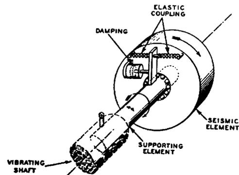
Figure 3.3 Torsigraph Mechanical Components (Draper<sup>6</sup>)
