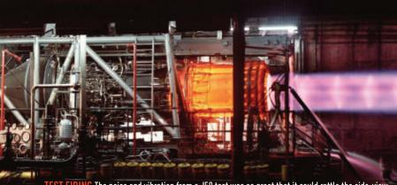
**TEST FIRING** The noise and vibration from a J58 test was so great that it could rattle the side-view mirror off nearby cars. The engine was developed at an isolated research center in Florida.
