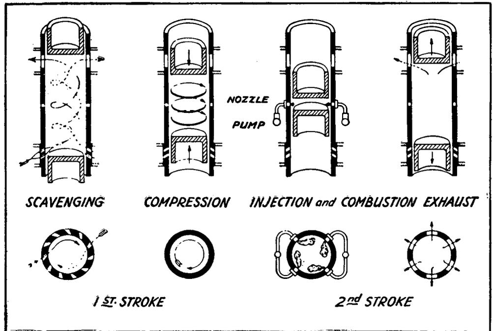
Fig. 36.—Functioning of piston-controlled ports.
