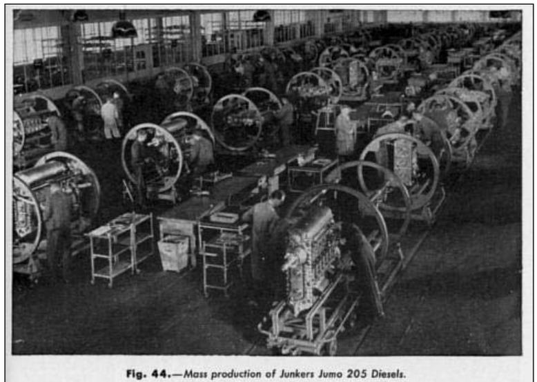
Fig. 44.—Mass production of Junkers Jumo 205 Diesels.
