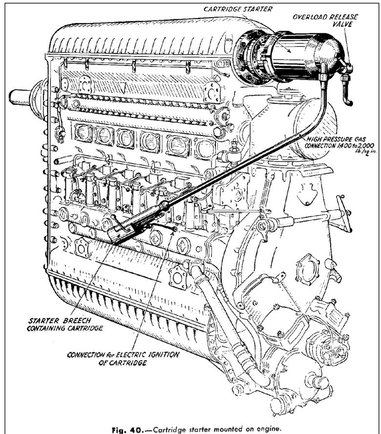
Fig. 40.—Cartridge starter mounted on engine.
