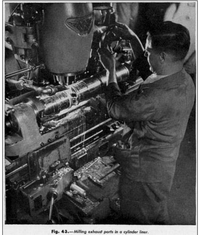
Fig. 43.—Milling exhaust ports in a cylinder liner.
