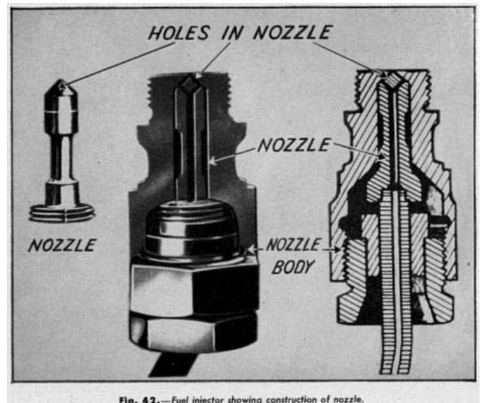
Fig. 42.—Fuel injector showing construction of nozzle.
