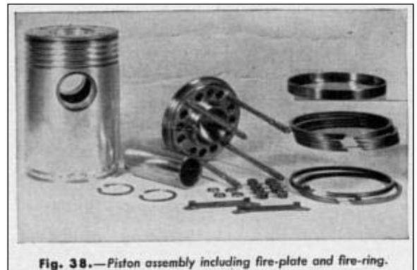
Fig. 38.—Piston assembly including fire-plate and fire-ring.
