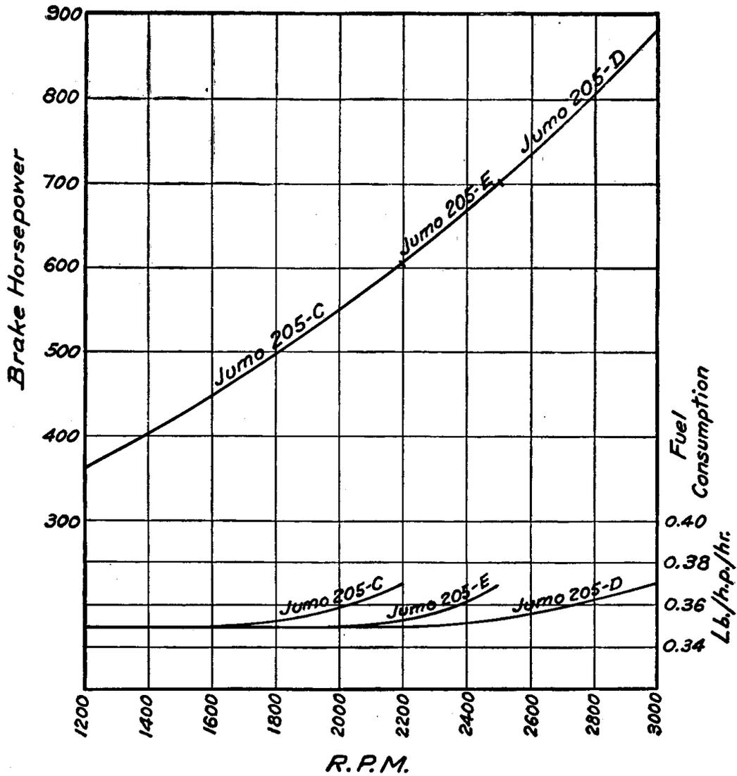
Fig. 46.—Power and fuel consumption curves.
