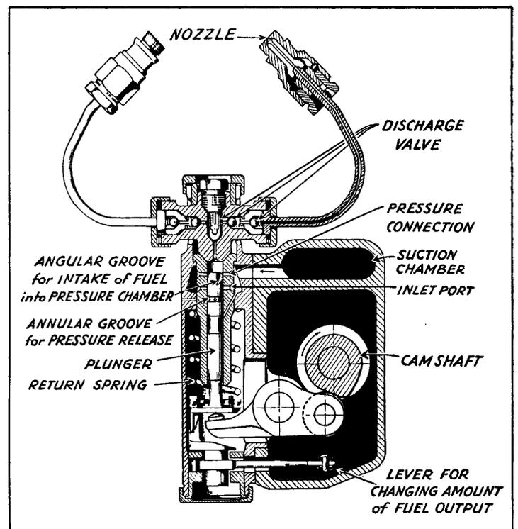
Fig. 41.—Junkers fuel injection pump and its two injectors.
