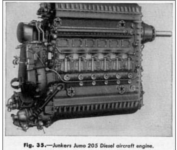
Fig. 35.—Junkers Jumo 205 Diesel aircraft engine.
