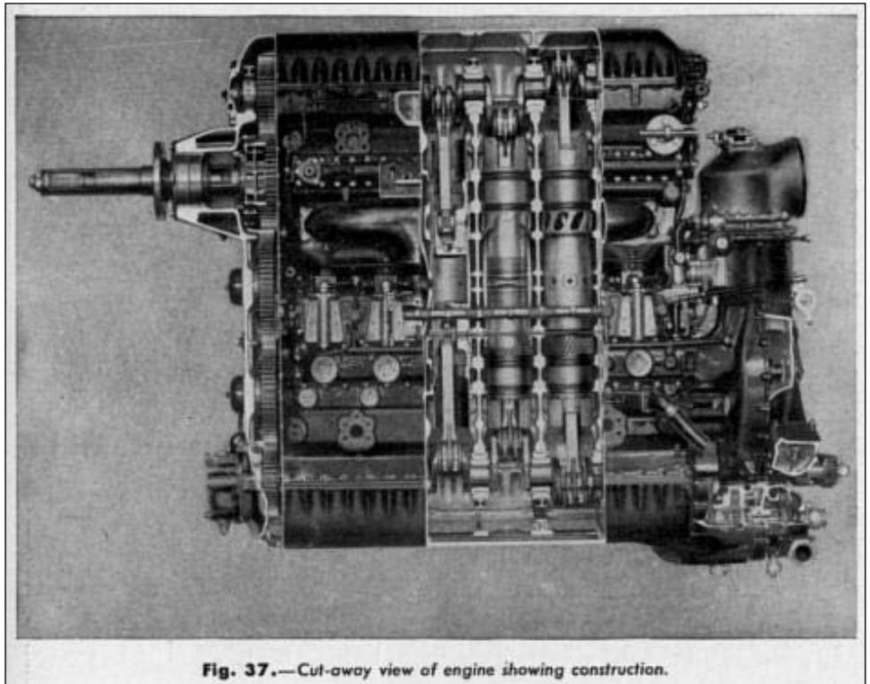
Fig. 37.—Cut-away view of engine showing construction.
